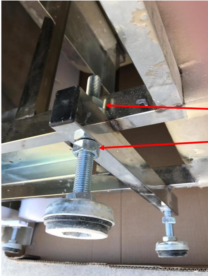
Feet adjustment – Each feet/leg can be adjusted up or down, as required independently to allow for a 100% water level installation.
